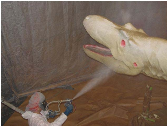
GlasCraft Probler P2 gun in use on a Streamline design
